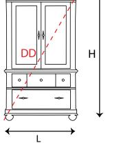
Case goods diagonal depth DD must be less than the entryway dimension 1, stairway dimensions 3, 4 & 8 and all interior doorways 6 or 7.
