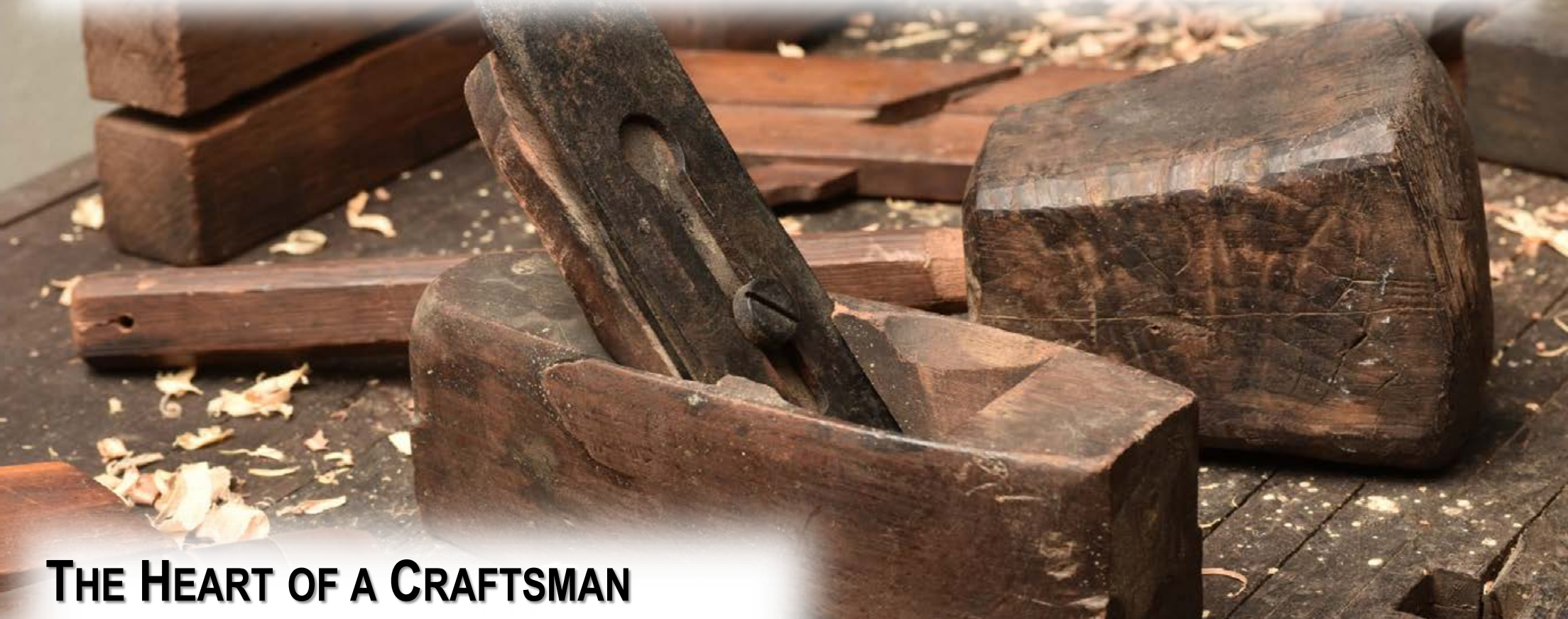
Picture: Hand Plan and Wooden Hammer Hand Planes are used to smooth out wood and Hammers are used to help assemble Mortise and Tenons
